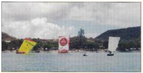
The sail is a large rectangle, and the boom runs from what would be the gooseneck and tack up to the upper comer of the sail opposite the mast. A sheet is attached to the end of the boom and another to the loose-footed clew.
